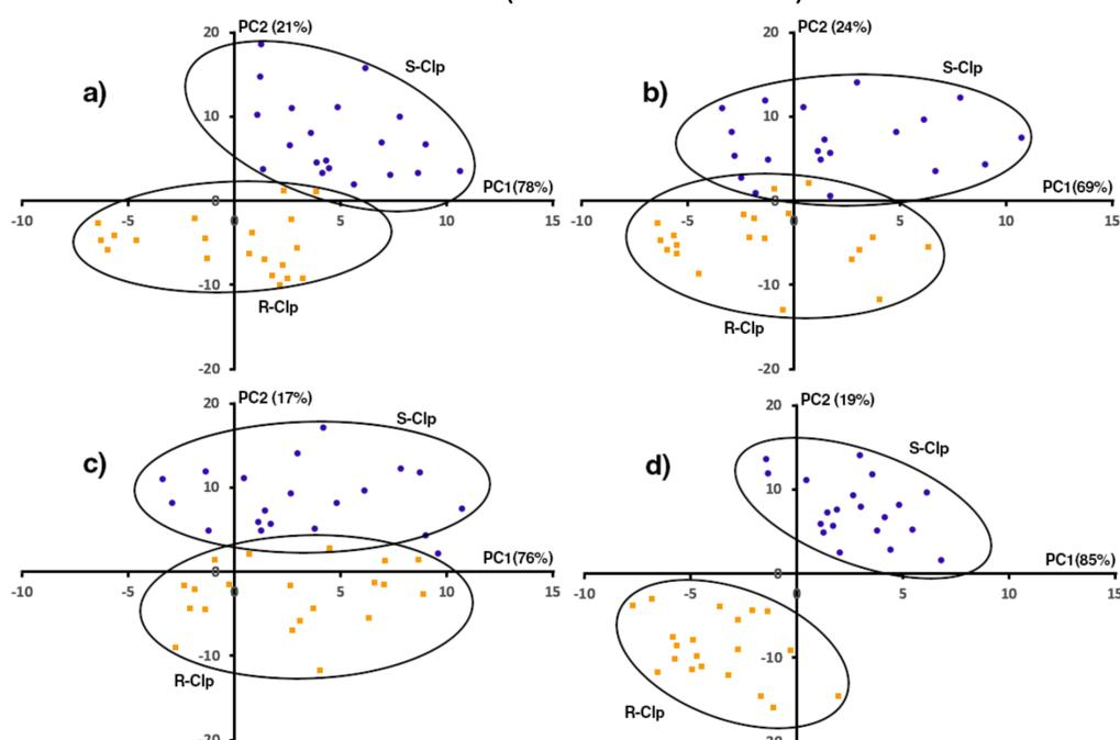
Score plots of the PCA-modeling of the DPVs of Clp enantiomers obtained using GCE/CpX/CPD1 (a), GCE/CpX/CPD2 (b), GCE/CpX/CPD3 (c) and the sensor system (d).
