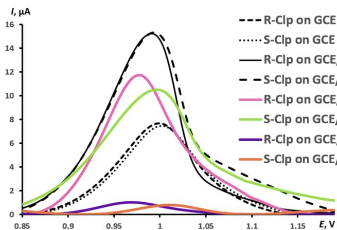
Differential-pulse voltammograms of clopidogrel enantiomers on various electrodes (concentration 0.5 mM)
