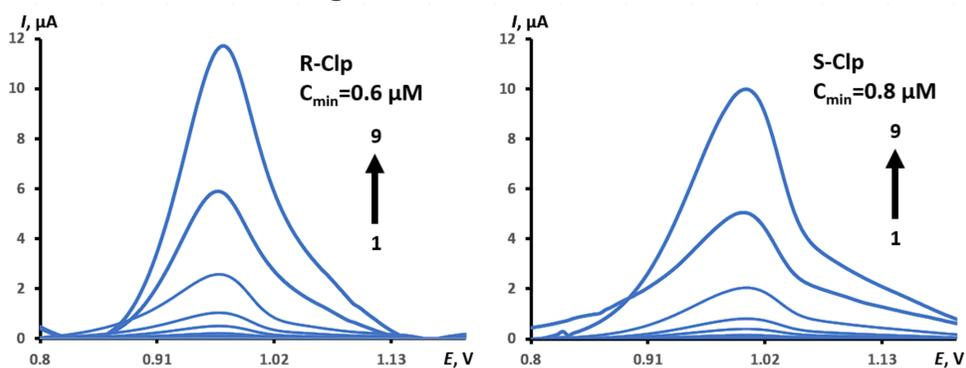
Concentration dependences of enantiomers of clopidogrel on the developed sensors (concentrations 1-9: 0.001, 0.0025, 0.005, 0.01, 0.025, 0.05, 0.1, 0.25, 0.5 mM)
