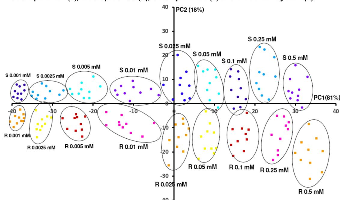
Score plots of the PCA-modeling of the DPVs obtained using the sensor system with different concentrations of Clp enantiomers
