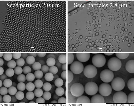
Change in seed particle size influences the size of the resulting particles (larger seeds lead to larger particles), but neither shape nor morphology differ significantly.
