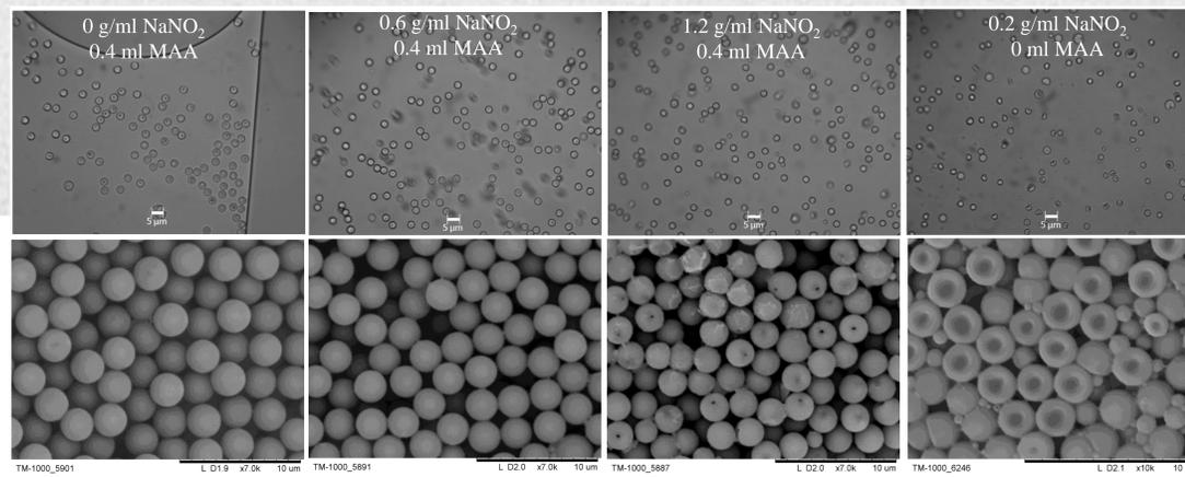
Increase in inhibitor concentration ( $\text{NaNO}_2$ ) leads to no significant change in particle size. However, there is an increase in the concentration of carboxyl surface groups, indicating the incorporation of higher amounts of MAA. The increase in  $\text{NaNO}_2$  concentration also influences the formation of defects within the polymer microspheres, which become more pronounced with higher inhibitor concentrations.
