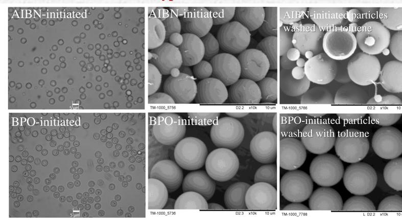
Given that AIBN is more water soluble than BPO ( $10^{-2}$  wt. % for AIBN,  $10^{-4}$  wt.% for BPO), it is plausible to suggest that the polymerization primarily takes place at the surface of the particles, resulting in the formation of a shell structure around the polystyrene seed microsphere. When exposed to toluene, the shell can crack, leading to the removal of polystyrene core from the center and the formation of hollow, half-spherical shells.
