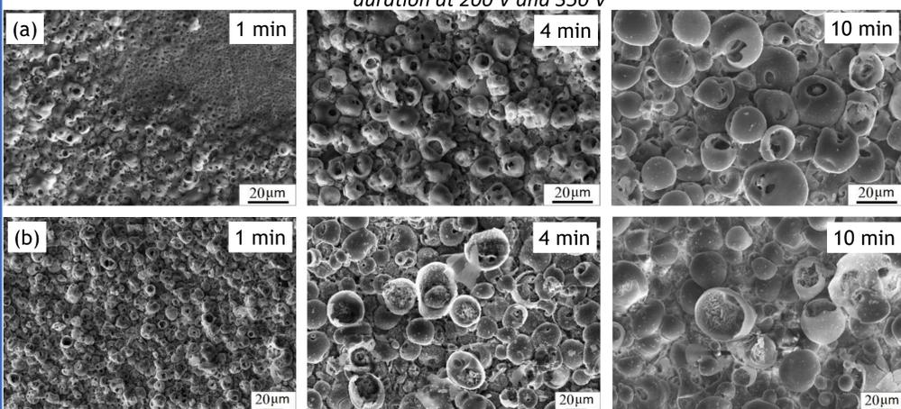
FIG. 2 SEM-images of the coating surface deposited at 200 V (a) and 300 V (b) with different duration.
