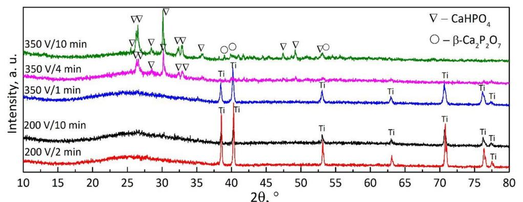
FIG. 4 XRD patterns of CaP coatings deposited at different voltages with different duration
