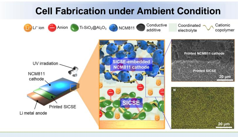
✓ The SSLMB full cell was featured with the seamless integration of the Li metal anode, printed SICSE, and printed NCM811 cathode.
