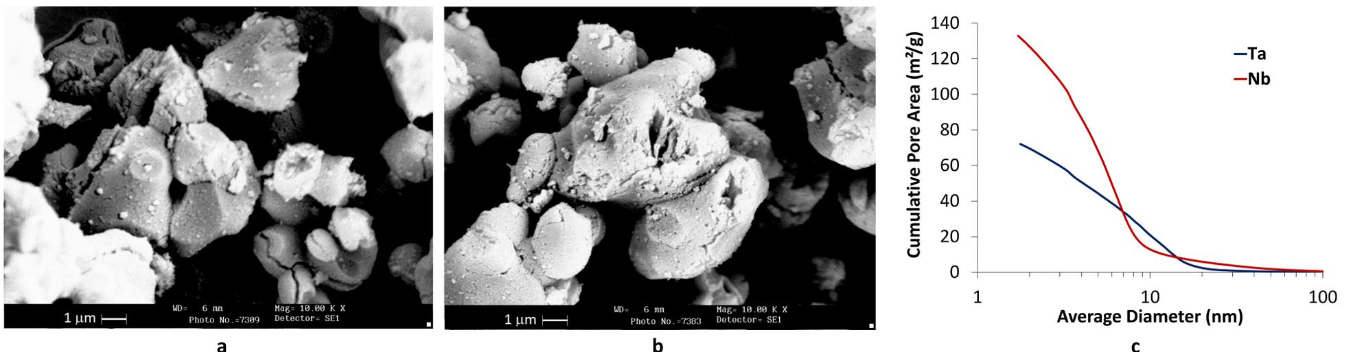
Fig. 3 – Microphotographs of (a) Tantalum ( $S=70 m^2/g$ ) and (b) Niobium ( $S=130 m^2/g$ ), and (c) BJH Desorption Cumulative Pore Area (Larger)
