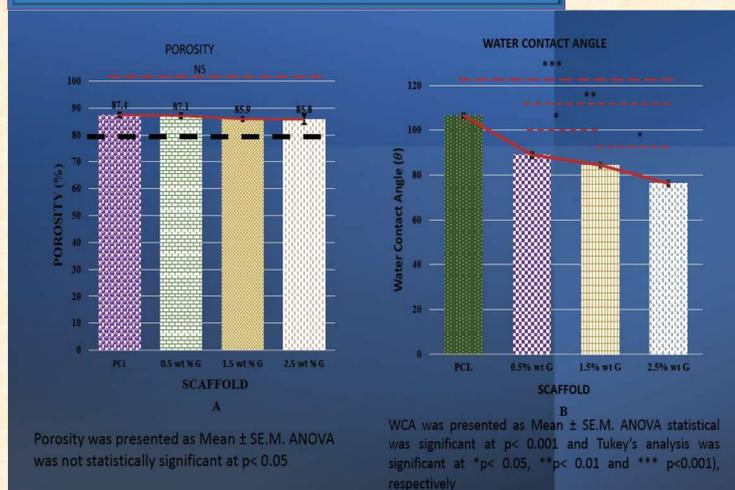
In this study, the total porosity of the scaffolds was determined using a liquid displacement method. The structures had a total porosity of more than 85%. When compared to the cancellous scaffolds (average porosity 79.3%), the porosity of the scaffolds is ideal (A).<sup>(2,3)</sup>
