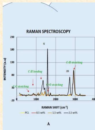
With increasing graphene content, the PCL peaks become less apparent as the intensity of the graphene's characteristic D (1350 cm<sup>-1</sup>) and G bands (1620 cm<sup>-1</sup>) increases, leaving only the D and G band graphene peaks visible. The ratio of the graphene D and G band intensities (I<sub>D</sub>/I<sub>G</sub>) falls marginally with increasing graphene content. This is because the composite's crystalline size decreases as the graphene content increases (A).<sup>(5,6)</sup>
