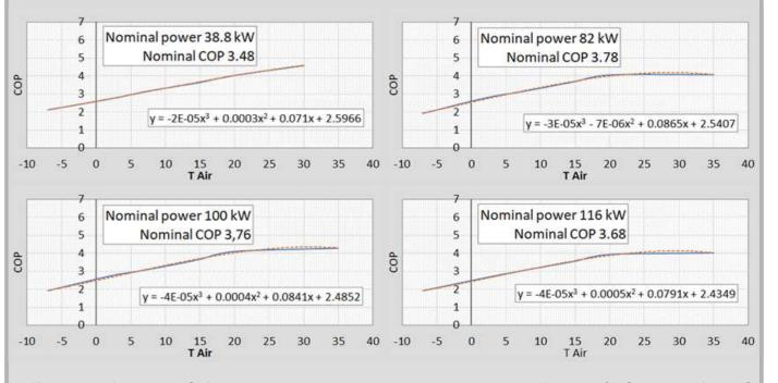
The analysis of heating requirements was evaluated for each of the buildings using hourly dynamic simulations carried out by the commercial tool Termolog. After the evaluation of the thermal requirements as previously described, commercial heat pumps were chosen for each building analysed. The size of the heat pump has been chosen based on the design thermal load.
