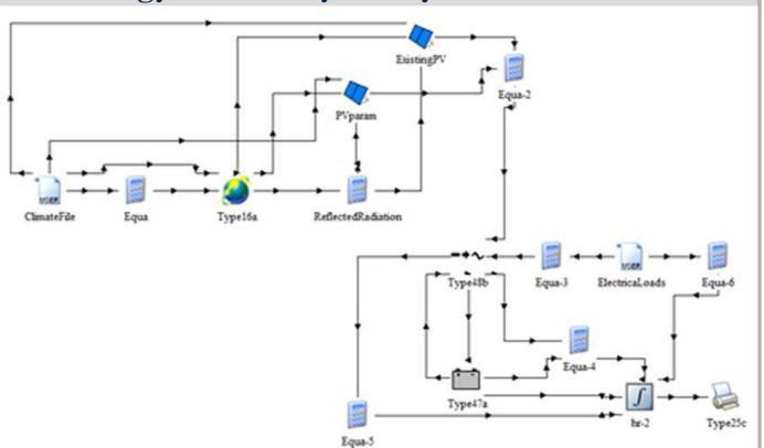
For the energy simulation an integrated approach in TRNSYS software was developed. This software does not include urban modelling and for this reason, Type9c was used, a data reader that considers the previously evaluated electrical loads. The simulations were carried out with a time step of 1 minute, but with the Quantity Integrator the results were printed directly with a monthly step to allow easier evaluations.
