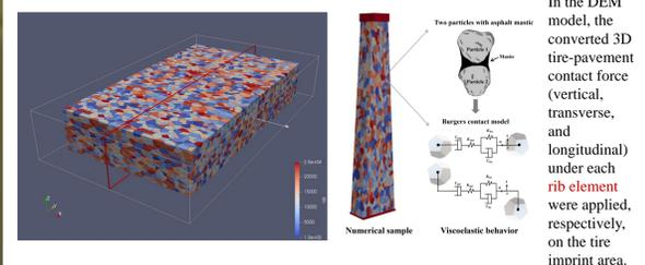
Particle displacement at two loading conditions
