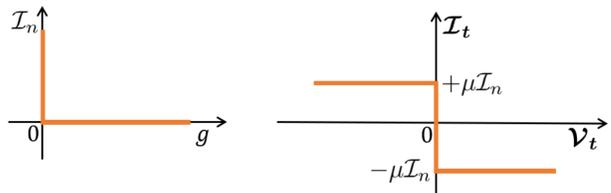
CD method: Contact formulation at velocity level
