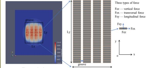
The contact stresses were converted into the equivalent concentrated forces using element shape functions of the FEM calculation. The bottom boundary of the DEM layer was fixed during the simulation.
