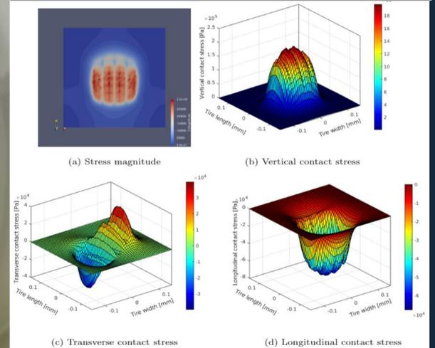
A drastic increase of the longitudinal contact stress occurs because of the braking force.
