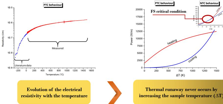
Evolution of the electrical resistivity with the temperature
