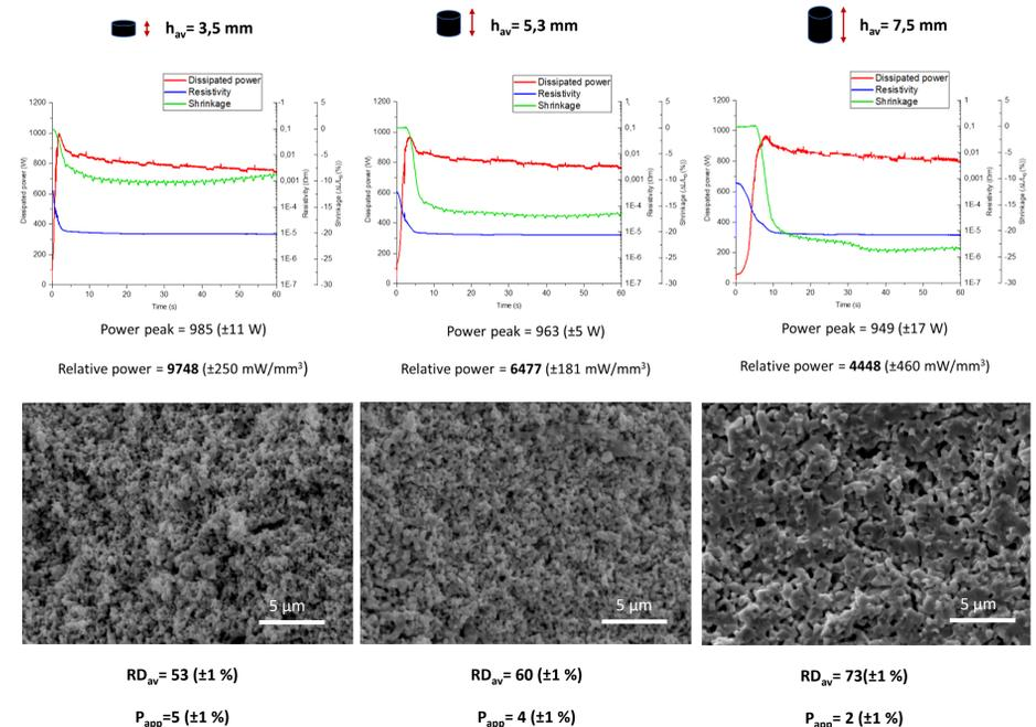
Differently from the expected results, a more intense relative power (mW/mm<sup>3</sup>) results in a much lower final density. Larger initial volume influences the time-scale of the resistivity evolution, resulting in a different time available for densification.
