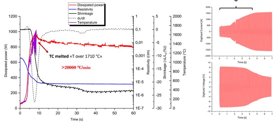
The WC pellet is sintered under 4 MPa and with a current limited to 2000 A.
