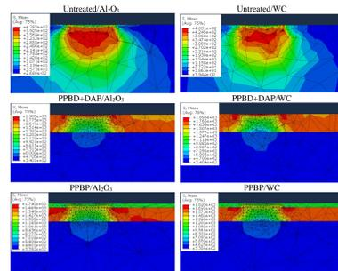
Figure 2. Von Mises stress distribution along the cross-section of the samples with Al<sub>2</sub>O<sub>3</sub> and WC tribo-pairs.
