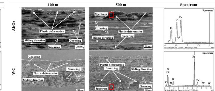
Figure 8. SEM-EDS micrographs of the wear track generated by the Al<sub>2</sub>O<sub>3</sub> ball and WC on untreated AISI 1018 steel under 5 N of load at a distance of 100 and 500 m at different magnifications.
