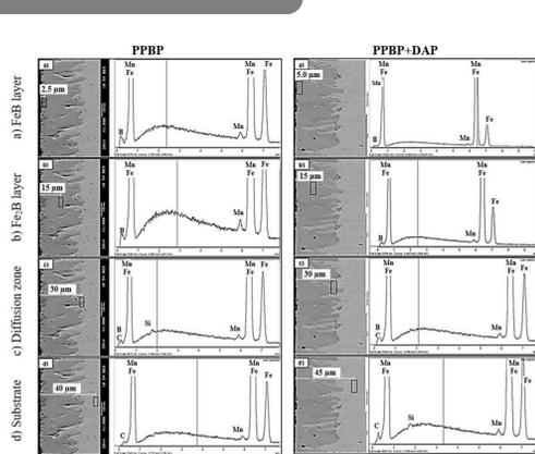
Figure 2. SEM-EDS spectrum in cross-section obtained for PPBP, and PPBP+DAP.
