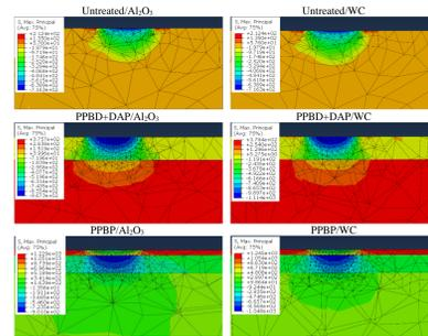
Figure 3. Principal stress distribution along the cross-section of the samples with Al<sub>2</sub>O<sub>3</sub> and WC tribo-pairs.
