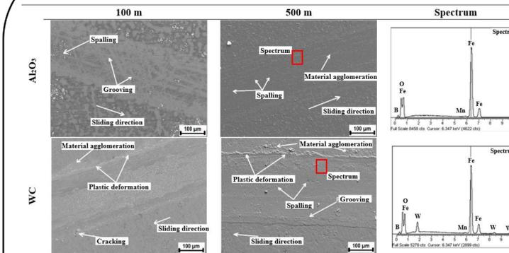
Figure 6. SEM-EDS micrographs of the wear track generated by the Al<sub>2</sub>O<sub>3</sub> and WC ball on PPBP 1018 AISI steel under 5 N of load at a distance of 100 and 500 m at different magnifications.
