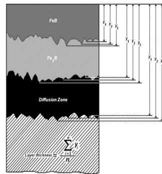
Figure 1. Representation of the formation of iron borides and measurement.
