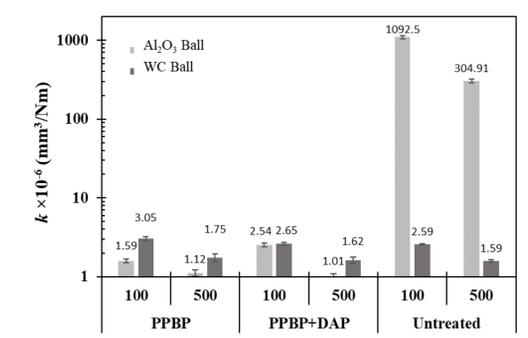
Figure 9. Specific wear rate (k) values for the overall experimental set conditions.
