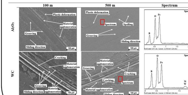
Figure 7. SEM-EDS micrographs of the wear track generated by the Al<sub>2</sub>O<sub>3</sub> ball and WC on PPBP+DAP AISI 1018 steel under 5 N of load at a distance of 100 and 500 m.
