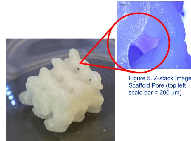
Figure 4. 3D Printed Bone Scaffold
