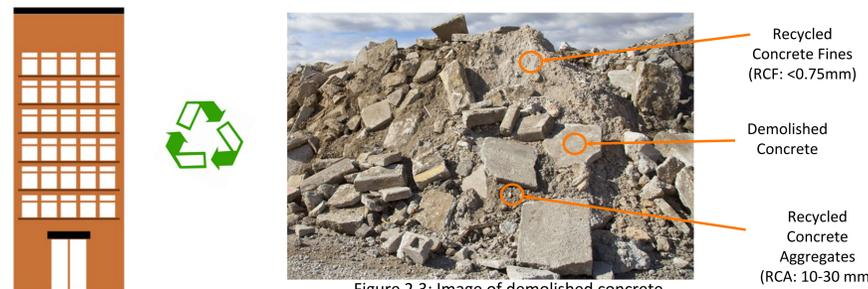
Figure 2.3: Image of demolished concrete
