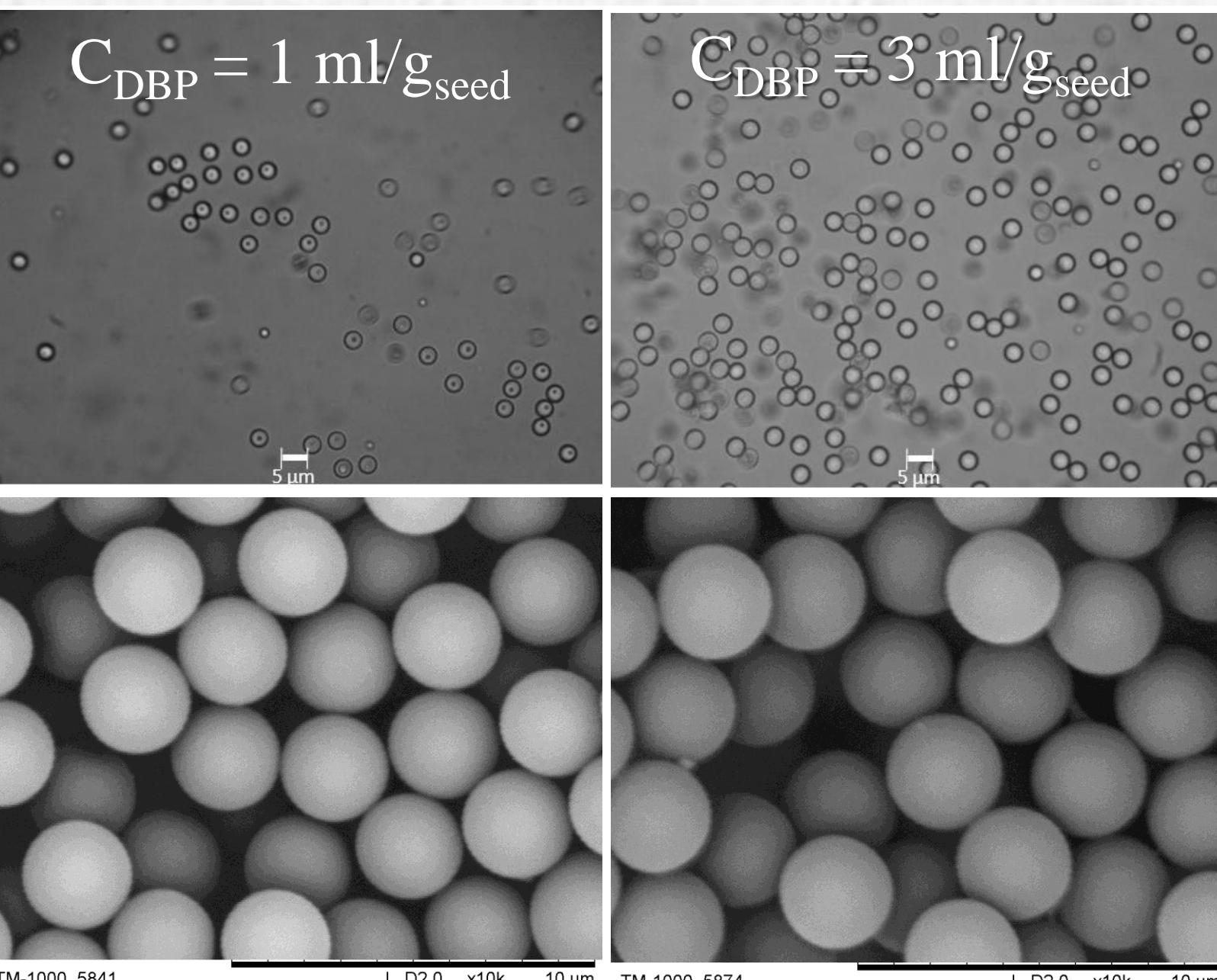
The median particle size increases with the DBP concentration. In addition, the particle morphology also changes. At lower DBP concentration, there is a defect in the interior particle structure observed in the optical microscopy images. This may suggest a more homogeneous distribution of the monomer phase inside the particle, due to the larger amount of monomer introduced, diffusion of which is facilitated in the presence of larger amounts of DBP.
