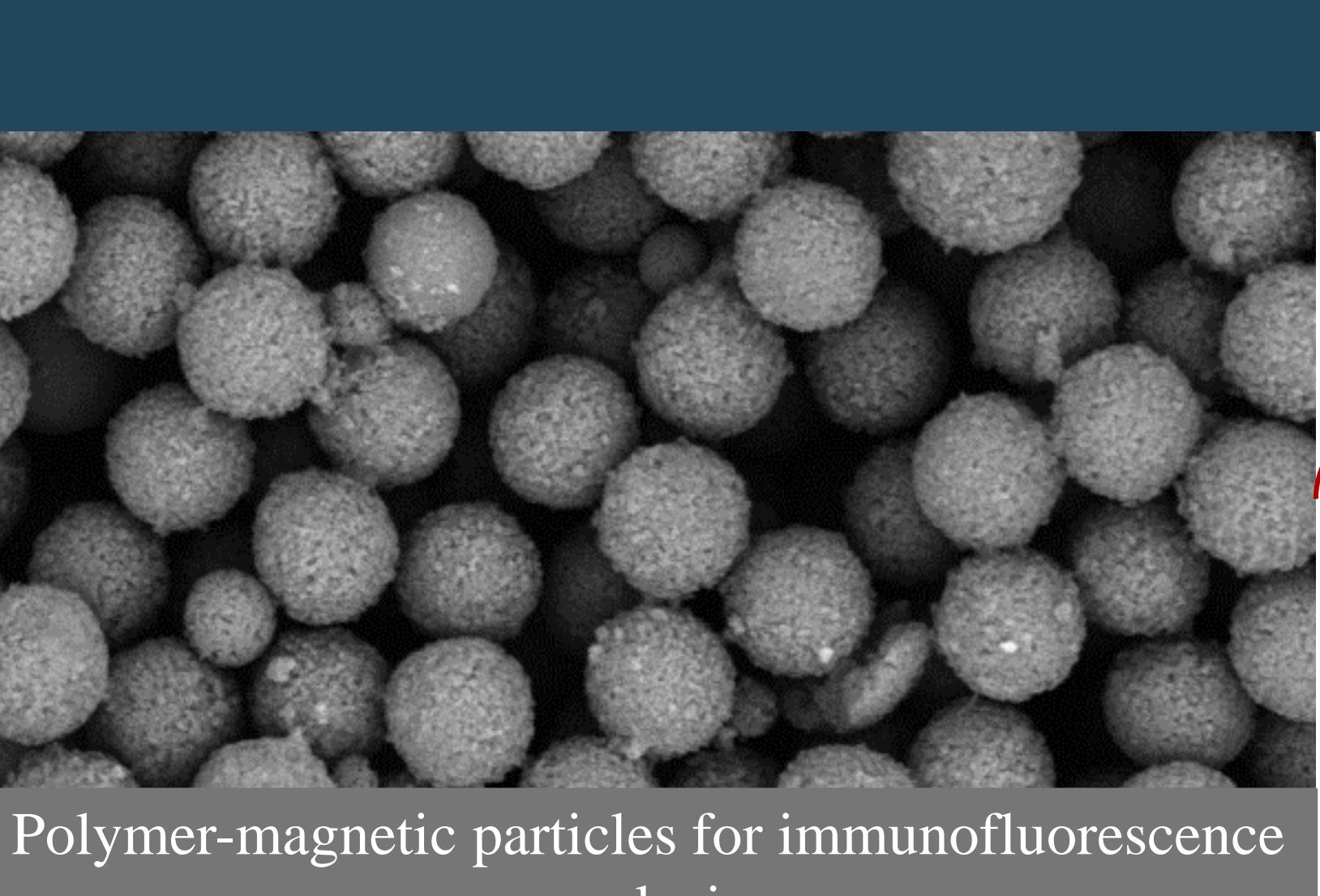
Polymer-magnetic particles for immunofluorescence analysis
