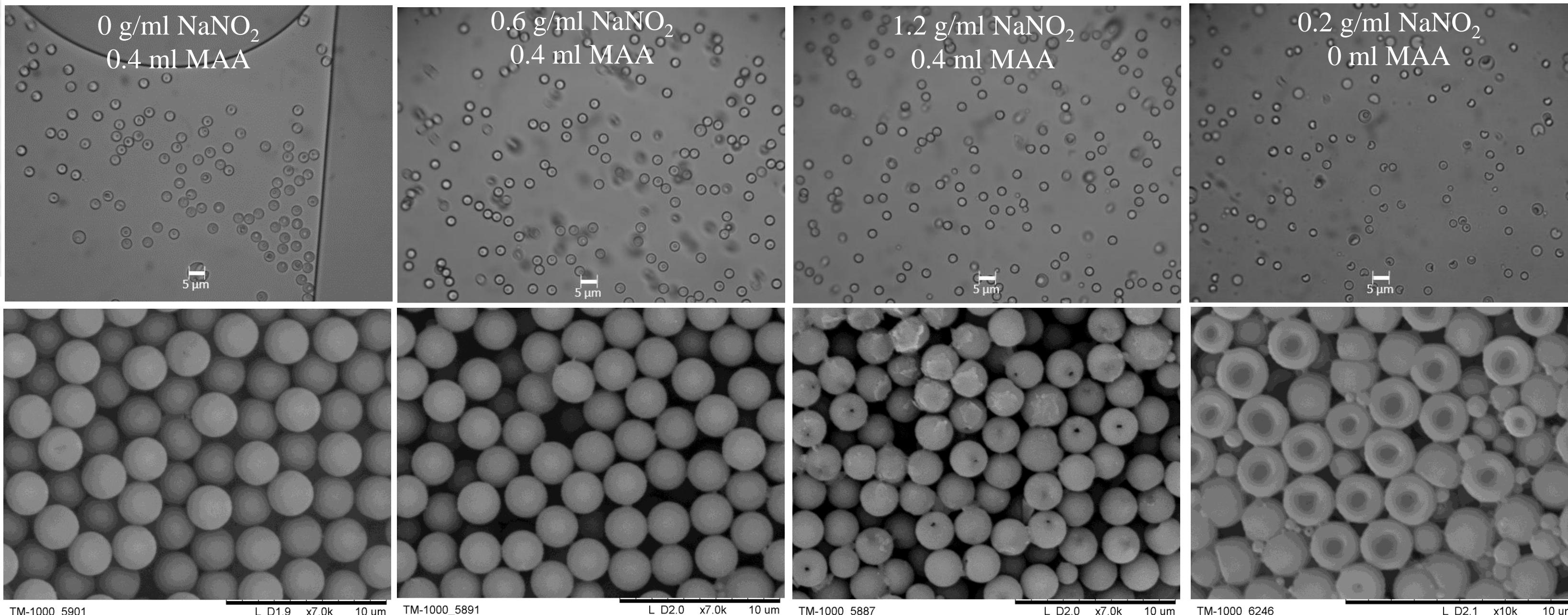
Increase in inhibitor concentration ( $\text{NaNO}_2$ ) leads to no significant change in particle size. However, there is an increase in the concentration of carboxyl surface groups, indicating the incorporation of higher amounts of MAA. The increase in  $\text{NaNO}_2$  concentration also influences the formation of defects within the polymer microspheres, which become more pronounced with higher inhibitor concentrations.
