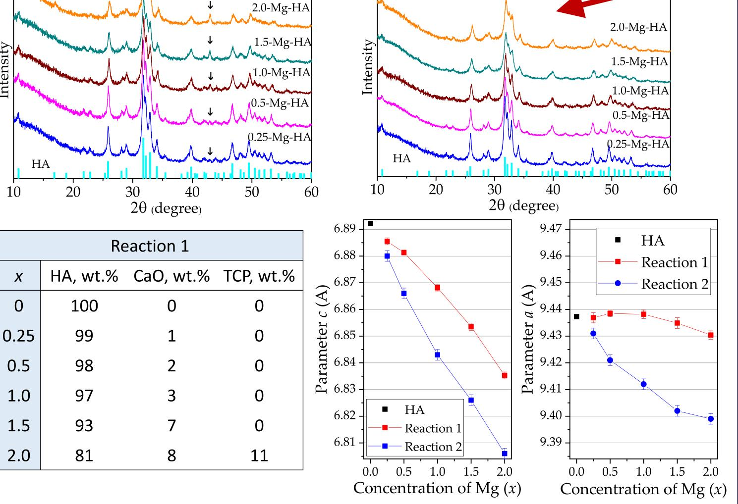
It has been established that, starting from the concentration x = 0.25, the samples synthesized with the introduction of magnesium oxide (reaction 1) contain the phase of the unreacted MgO reagent. However, the lattice parameters of the HA phase in these samples decrease with an increase in the concentration of introduced magnesium. This indicates only a partial incorporation of magnesium ions into the HA structure.
