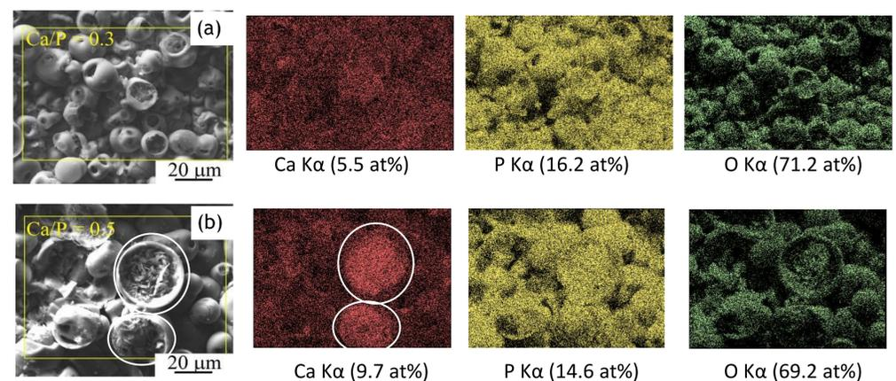
FIG. 3 SEM-images of the coating surface and EDX maps of the Ca, P and O distribution in the coatings deposited at 200 V (a) and 300 V (b).
