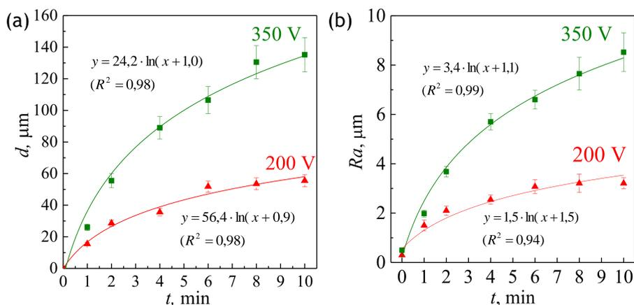
FIG. 1 Graphs of the coating thickness (a) and roughness (b) against the MAO duration at 200 V and 350 V
