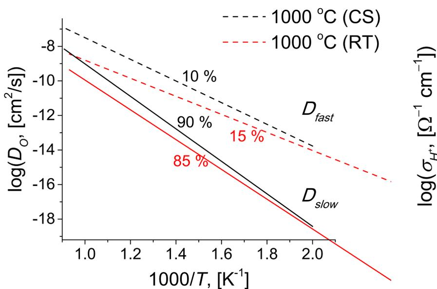
Fig. 1. Arrhenius plots for oxygen tracer diffusion coefficient for  $\text{PrNi}_{0.5}\text{Co}_{0.5}\text{O}_3$  sintered by conventional (CS) and radiation-thermal (RT) sintering at 1000  $^\circ\text{C}$  [2].
