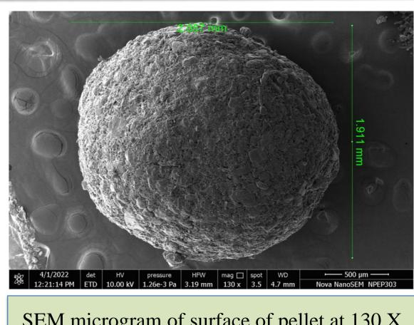
SEM microgram of surface of pellet at 130 X
