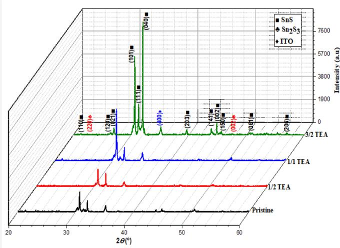
TEA has no significant effect on lattice parameters. However, it decreases the crystallites size. The (040) direction is unfavorable for SnS films since it limits the charge transport.
