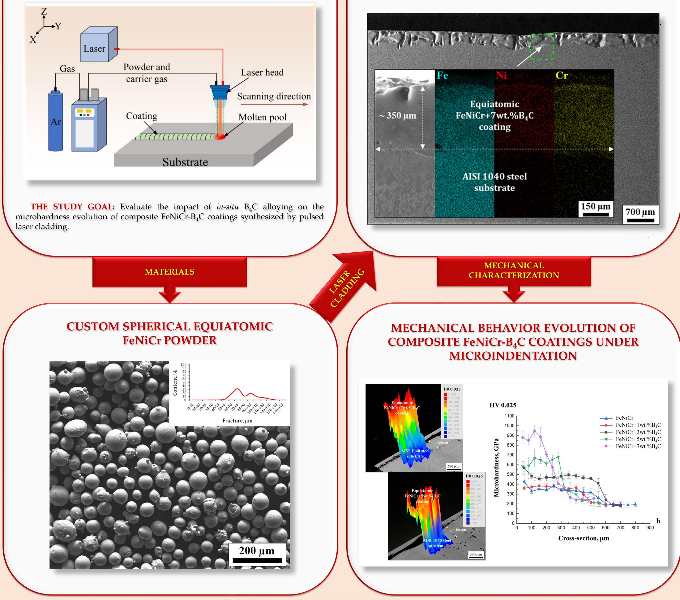
**ELEMENTAL MAPPING OF THE SUBSTRATE-COATING AREA ON THE CROSS-SECTION OF THE** FeNiCr+7wt.%B<sub>4</sub>C SAMPLE
