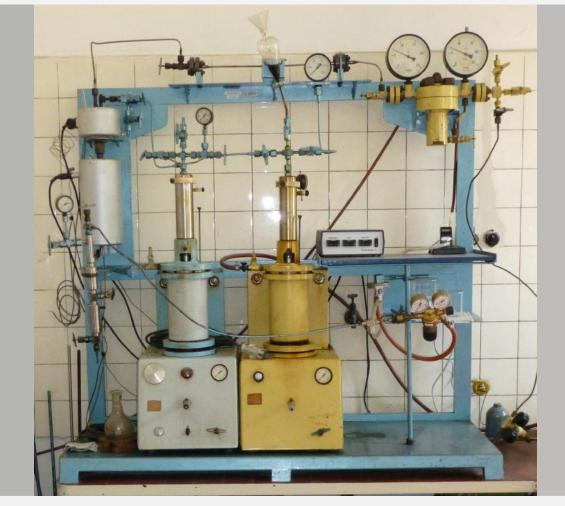
We started studying hydroprocessing around 1990. The first hydroprocessing unit was manually operated and equipped with a two-heating zones furnace. A pair of heavy piston pumps was used for the feedstock injection. The unit was not connected to PC and remote control was not, therefore, possible.
