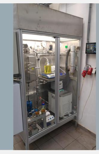
During the unit modernization, a four-heating zones furnace was implemented, control software was upgraded, the remote control was allowed, and the feedstock pump was modified for low flow rates and viscous feedstocks. The unit was jacketed and connected to the ventilation.
