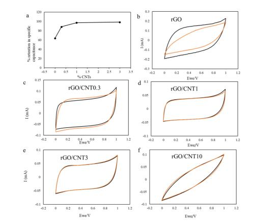
Percentage retention of specific (a) capacitance with respect to % of CNTs. (b) Cyclic Voltammetry in rest (black) and bend (orange) states at bending curvature of 90° in Na<sub>2</sub>SO<sub>4</sub> electrolyte.
