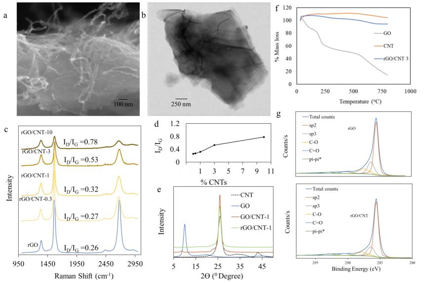
(a) SEM (390kx) image of rGO/CNT-1 (b) STEM image of rGO/CNT-1 Raman Spectroscopy of laser-reduced rGO/CNT-1.  $(d)I_D/I_G$  ratio (C) dependence with the number of CNTs. (e) XRD of GO/CNT-1 films. (f) TGA of rGO, CNT and rGO/CNTs. (g) XPS of rGO and rGO/CNT.
