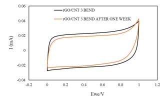
Long term stability of composite showing 88.36% retention 111 specific capacitance.
