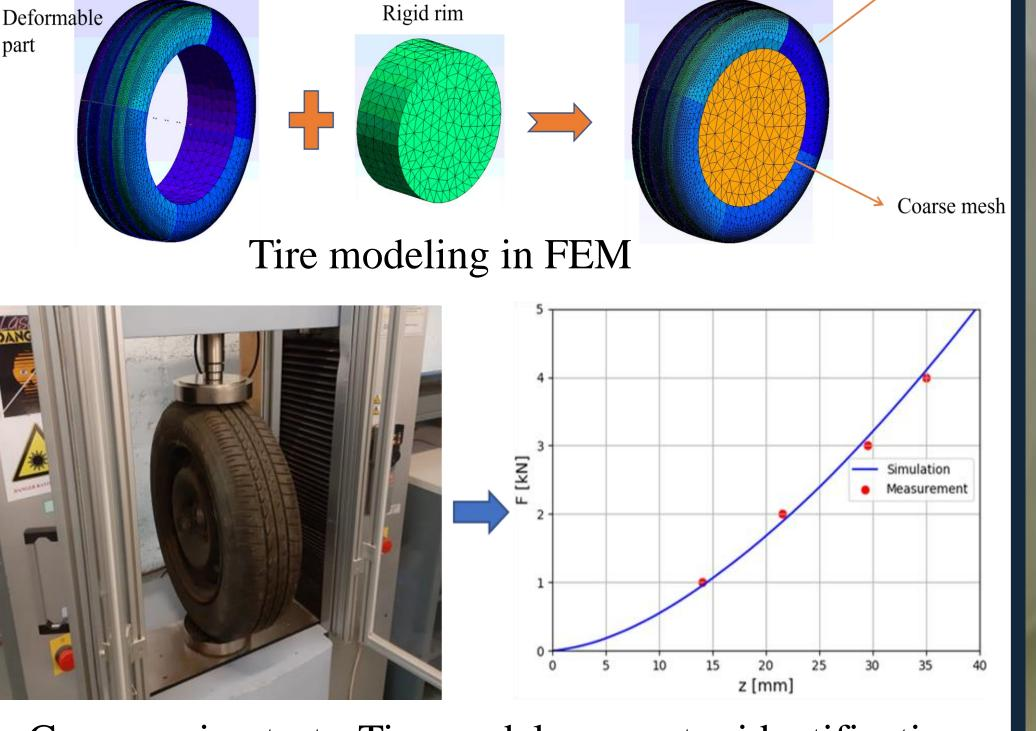
Compression test - Tire model parameter identification
