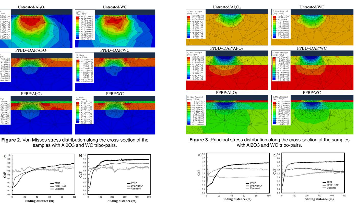
Figure 4. CoF against the relative wear distances with an Al2O3 ball for a) 100 m and b) 500 m
