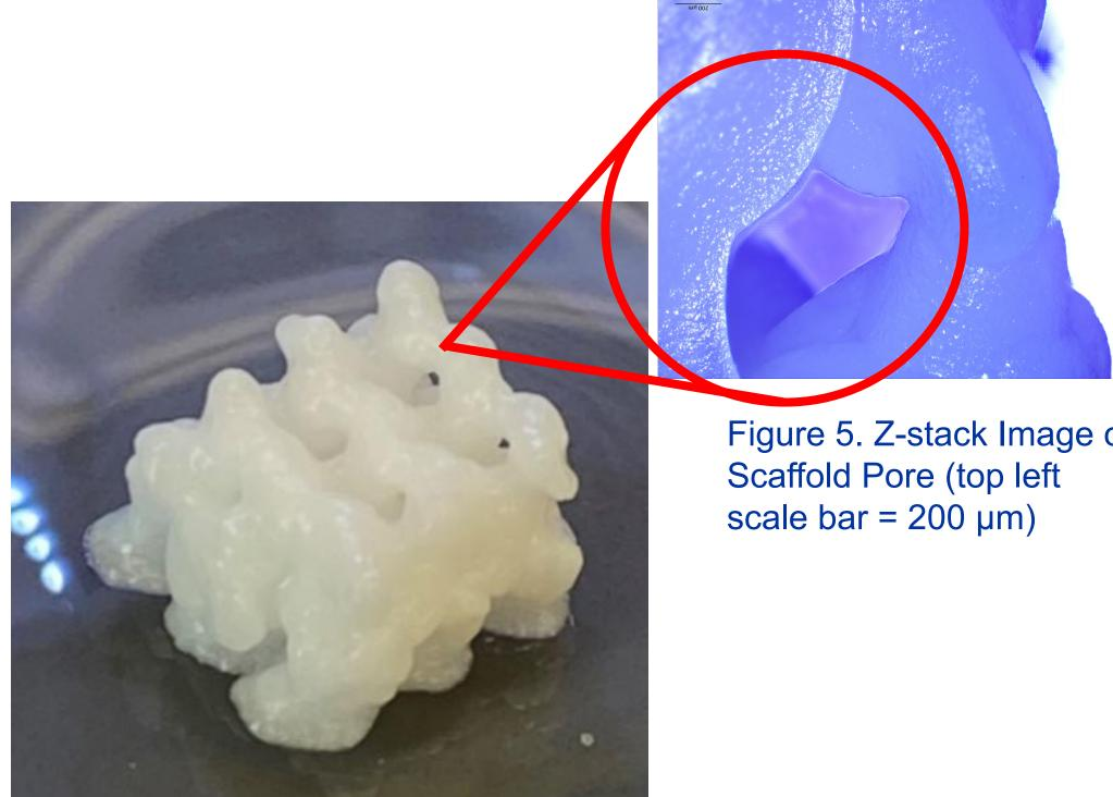
RESULTS • Average short diameter of pores: 821.33 µm • Average long diameter of pores: 1299.01 µm • PBS destroys chemical cross linked prints\*
