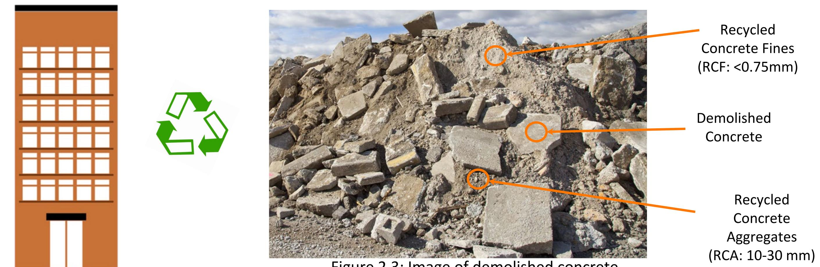
Figure 2.3: Image of demolished concrete
